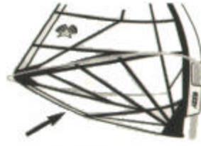
Foot is tight, outhaul correct
